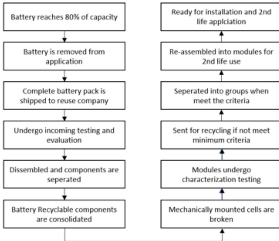
Figure 3: Remanufacturing process for B2U. Adapted from (Hossain et al., 2019).
