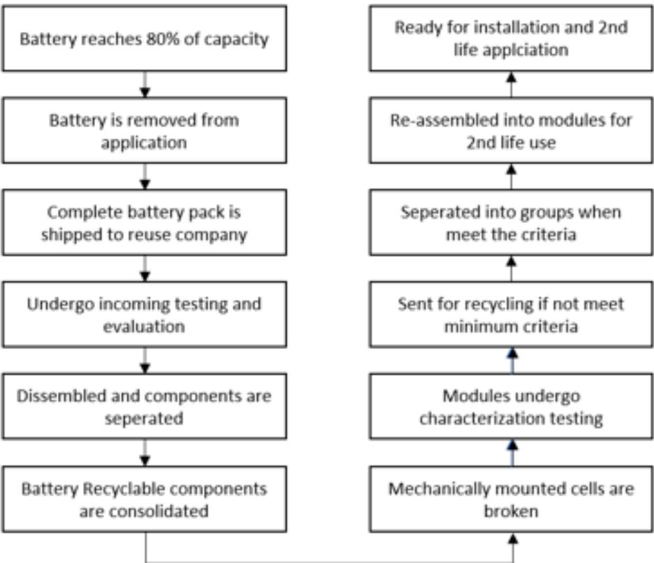
Figure 17: Remanufacturing process for B2U. Adapted from (Hossain et al., 2019).
