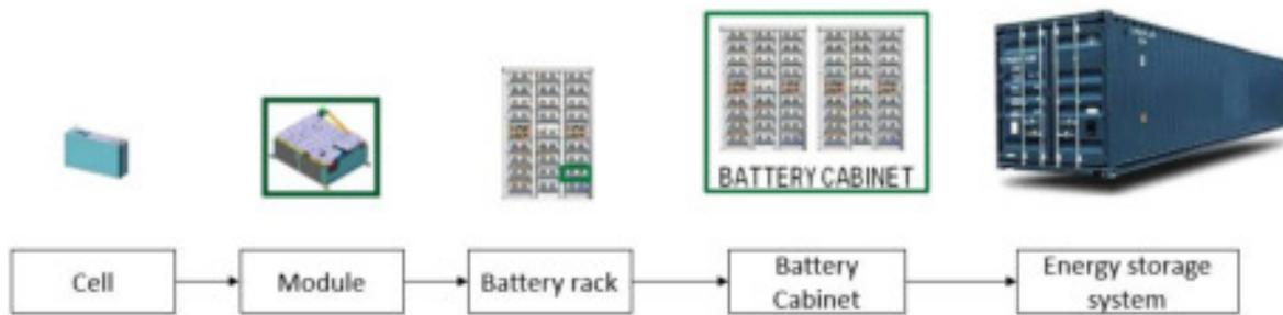
Figure 4: Steps from individual cell towards a BESS. Adapted from (Bowler, 2014).
