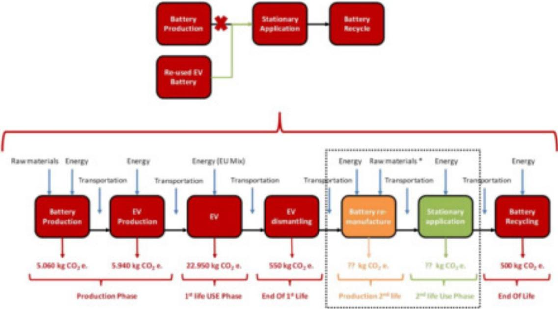
Figure 5: : Life Cycle assessment based on the CO<sub>2</sub>-emissions for B2U (Casals et al., 2017).
