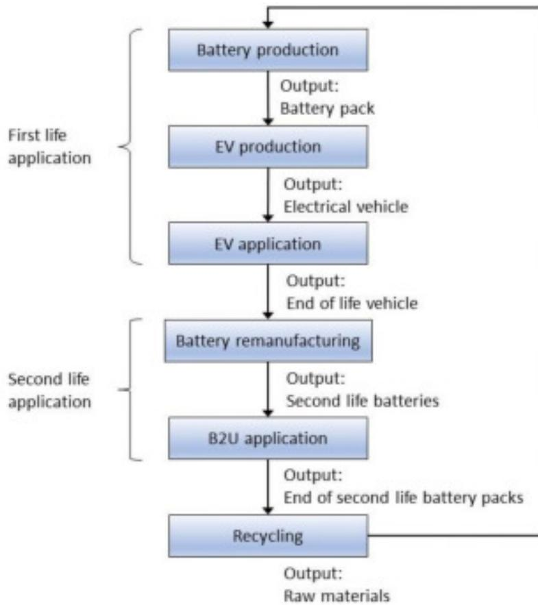
Figure 2: Value chain of battery second use. Based upon: (Casals et al., 2019; Neubauer & Pesaran, 2011; Reinhardt et al., 2019).
