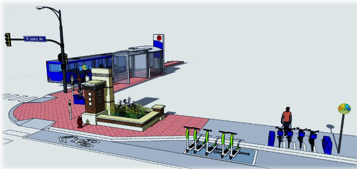
Figure 10: Example of a mobility hub including bus stop, e-scooters, and bike sharing 22
