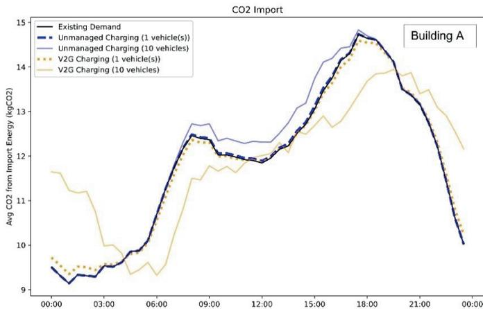
Figure 30: Carbon emissions imported for Building A
