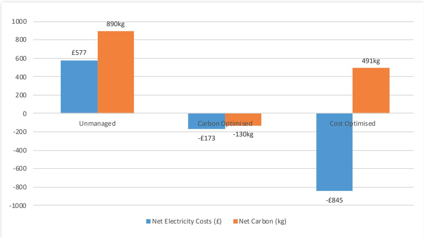
Figure 48: Cost & Carbon for UoW Site Runs with Dynamic Tariff
