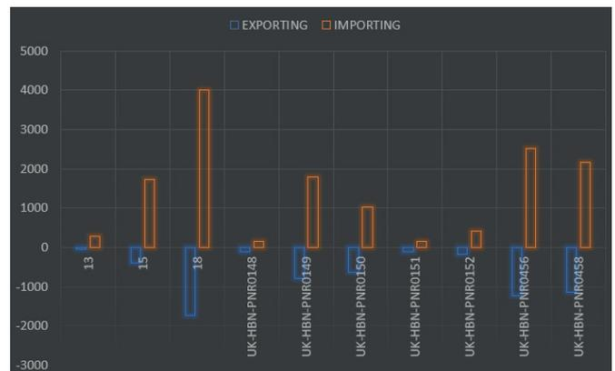
Figure 12: Import and export by charger in kWh
