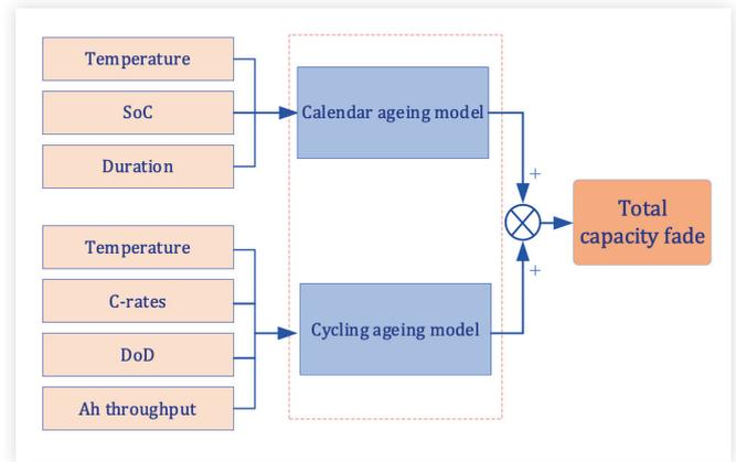
Figure 38: Combined degradation model framework
